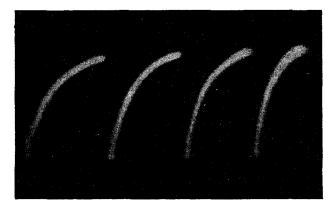
Fig. 37. This waveform is the result of applying the bias necessary to produce maximum amplitude of the sweep. Note the very definite bend in the charging portion of the cycle and the consequent non-linearity.
