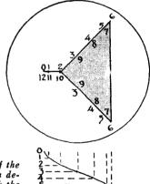
Fig. 386-D. The effect of over modulation of the modulated signal can be seen in the pattern developed. The sweep voltage is in phase with the modulated signal in this instance.
