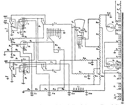
Schematic diagram of the Triumph Model 800 cathode-ray oscillograph. Note the two rectifiers, the type 879 supplying the high voltages for the cathoderay tube, type 906, and the type 80 supplying the bias and plate voltages for the remainder of the tubes.
