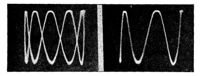
Fig. 101. A, left, B, right. Both patterns are of a 5-1 ratio. The one shown in B has its peaks coinciding.
