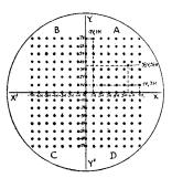
however, the voltage applied to the plates changed in very small increments, the spot would appear so close to the previous position that when recurrent at a rate, say 16 to 20 times per second, the entire active area would appear fluorescent.
