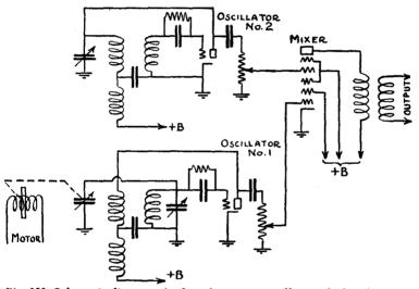
Fig. 252. Schematic diagram of a beat frequency oscillator which is frequency modulated by the motor driven variable condenser in the lower left corner of the diagram. This type of oscillator, when frequency modulated, provides a band width that is constant for any output frequency.
