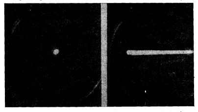
Fig. 65-C. Here the intensity control was too far advanced, this being evidenced by the halo around the spot. Fig. 66-C. The spot of Fig. 65-C shows a trace that is broad at one end and narrow at the other.
