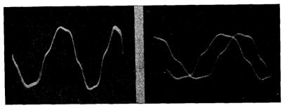
Fig. 81, left, Fig. 82, right. Even though the wave impressed on the vertical plates of the cathode-ray tube is distorted, as in Fig. 81, the same need for proper synchronization exists. Improper adjustment of the synchronizing control is responsible for the pattern of Fig. 82
