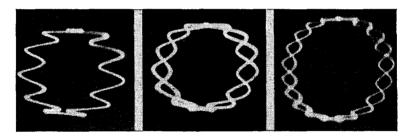
Fig. 121. A 10-1 ratio Fig. 122. A 13-2 ratio Fig. 123. A 19-2 ratio pattern. Compare Fig. pattern. pattern. 117.
