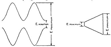
Figs. 382, left, 383, right. A modulated wave envelope showing amplitude modulation is shown in Fig. 382. A trapezoidal pattern showing the relation between the carrier amplitude and the audio signal amplitude is shown in Fig. 383.
