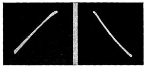
Fig. 95. A, left, B, right. Both patterns show a I-I ratio between the frequencies. The phase difference in A is 180° and that in B is 0°.
