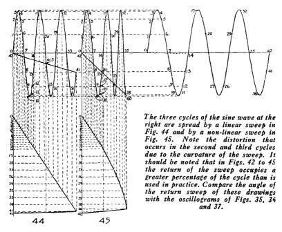
in from the position which is the start of the beam may be fairly true representations of the waveform voltage applied to the vertical deflection plates. The sweep voltage frequency in figures 42, 43, 44 and 45 has been kept constant and the voltage being observed has been changed in frequency. In practice to obtain a greater number of cycles upon the screen, for any one frequency input to the vertical deflection plates, the sweep frequency is changed.
