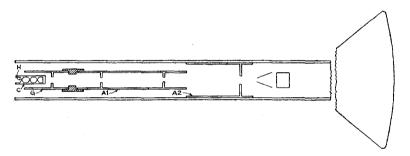
Fig. 4. In the sketch of the RCA type 906 tube the following letters indicate the various elements: H, the heater; C, cathode; G, shield grid; AI, first anode; A2, second anode. The two pairs of deflecting plates are to the right of A2. It will be noted that these plates are at an angle to the main axis of the tube. This arrangement of elements in a glass envelope or bulb constitutes what is sometimes referred to as an "electron gun."
