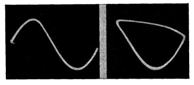
Fig. 79, left, Fig. 80, right. The proper amount of synchronizing voltage was applied to get the single cycle of Fig. 79. When the maximum amount of synchronizing voltage was applied, the distorted figure of Fig. 80 resulted.
