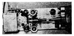
the "X" axis, but it is becoming more common to provide both centering controls. Figure 22 shows the spot positioning controls' locations on a commercial oscillograph.
