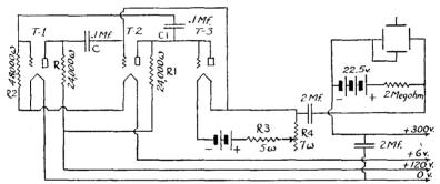
Fig. 39. Schematic diagram of the so-called multi-vibrator circuit. Note that this is nothing more than a two-stage resistance-capacity coupled amplifier arranged to feed back on itself. It is possible to generate fundamental frequencies up to 30 or 40 kilocycles.
