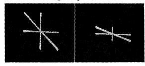
Fig. 93-C, left, Fig. 93-D, right. A phase difference of 0° exists between the two voltages. In C equal amplitudes on both axes give the pattern a 45° angle with the horizontal, but when the horizon-
