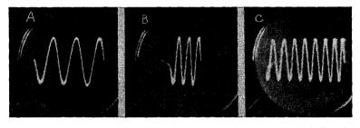
Fig. 68. The sweep amplitude of A is the same as that in Fig. 67-C, but the sweep frequency has been reduced so that three cycles appear on the screen. When the amplitude of the sweep is reduced, as in B, the peaks of the waves become sharp and make it difficult to get a true idea of the wave's khape. In C the sweep frequency has been further reduced with the result that the peaks are more pointed than in B.
