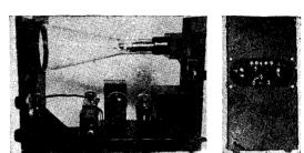
Photograph at left courtesy National Union Kudio Corp. Fig. 54. Left, panel of the National Union oscillograph. The cross-section lines are ruled on a transparent shield that clamps over the screen of the tube. Middle, chassis showing the 5-inch cathode-ray tube in position. Right, rear panel to which connections are made to the deflecting plates.
