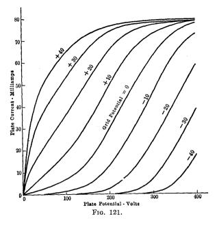
trol range the grid potential remains negative, and consequently the grid does not attract any electrons to itself, and no current flows in the grid circuit.
