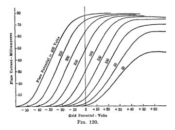
of the tube for the particular plate voltage and filament temperature (or current) used. Assuming the latter to be constant, a family of such curves is obtained corresponding respectively to various values of plate voltage, as shown in Fig. 120. The higher the plate potential, the more the curve is shifted to the left, without substantially altering its shape, particularly for the higher values of plate potential.
