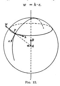
It will be noted that the energy vector is inversely proportional to the square of the distance r of the point P considered: the radiated energy, crossing in its outward motion successive concentric spheres of increasing radius, the surface area of which increases as the square of the radius (that is, as  $r^2$ ), and the energy per unit area of sphere surface decreases in inverse proportion to  $r^2$ .
