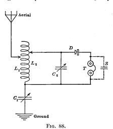
described, it is necessary that the high impedance of the telephone-receiver windings be shunted by a small capacity, or else the high-frequency oscillations will not reach the detector D, being choked out by the telephone-winding reactance. This small pass" condenser is shown here, the capacity between adjacent turns of telephone windings being, in most cases, sufficient for the purpose.
