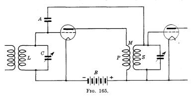
of the transformer M through which it is coupled to the following amplifier tube. When then an alternating current flows through the primary of the transformer G, an oscillation is set up in the circuit LC, alternately varying the grid potential of the tube T. This in turn varying the plate current of the tube, an amplified alternating electromotive force is induced in the secondary winding S of the transformer M, operating the following tube of the amplifier.
