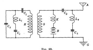
the stator and rotor windings, respectively, to external circuits of such inductance and capacity that, combined with the inductance of the alternator winding to which they are connected, they constitute oscillatory circuits resonating at the successive component frequencies.
