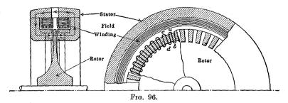
As an example of actual alternator construction, Fig. 96 represents schematically a small Alexanderson alternator. The
