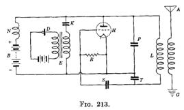
operation of the microphone D is impressed between the plate and filament of the tube H. A condenser K is connected in series with this secondary winding to prevent the direct current from the battery B flowing through it. The audio-frequency electromotive force thus varies the operating plate voltage of the tube, and correspondingly changes the amplitude of the high-frequency oscillations generated by it in the circuit PTL and in the antenna circuit.
