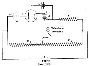
batteries B and C. The system being connected to a supply of alternating current of audible frequency, the bridge is balanced to make the telephone receiver silent, when the differential resistance of the tube is equal to
