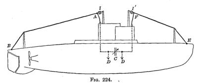
the surface. The maximum depth at which the signals are readable is dependent upon the wave length of the transmitting station. This depth increases with the wave length, and is about 21 ft. (for the top of the loop) when receiving signals of 10,000-m. wave length. The receiving apparatus used in these tests comprised a vacuum tube detector and three-stage resistance coupled vacuum tube cascade amplifier.
