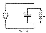
neglecting all resistances, the condenser current  $I_c$  and inductance coil current  $I_L$  are equal to
