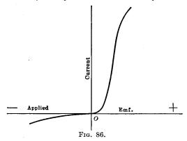
of the curve that the current flowing during the negative half of the cycle is negligible as compared to that flowing during the positive half-cycle, and rectification of the current is thus achieved.
