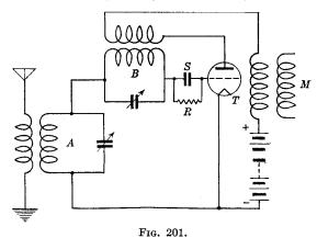
frequency electromotive force at the secondary terminals of the output transformer M.
