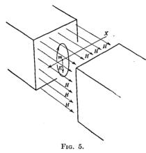
figure, from which it is seen that the magnetic force developed by the charge is, at some points, in the same direction as the lines of magnetic force H of the magnet (points located, in the figure, around the upper portion of the circle), and at other points (the lower portion of the circle) in opposite direction. In accordance with the pre-
