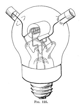
the tube. This type of tube, made in small size, is well adapted to the reception of short waves. In larger sizes, it may be used for transmitting purposes with several hundred volts on the plate, sometimes as many as 1,000 volts.
