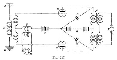
modulator, which is to eliminate the carrier-frequency current from the output circuit.
