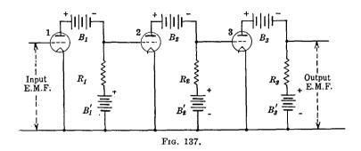
The resistance-battery coupled amplifier may be simplified by splitting the plate-circuit energizing batteries of the tubes in such manner that one part of these batteries may at the same time serve as grid-coupling batteries, as shown in Fig. 137, or even by using a single coupling battery, as in Fig. 138, which is derived from the arrangement of Fig. 137.
