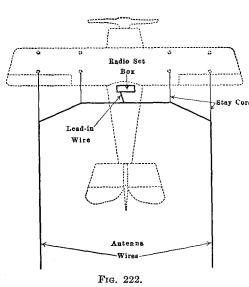
squadron flying or intercommunication between airplanes. Also, each of the trailing wires is only 150 ft. long, instead of the usual 300 ft. of the single wire antenna. This permits a greater liberty of flying, and enables the airplane
