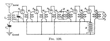
rent induced in the detector circuit by the plate current of the tube  $A_3$  will flow through the secondary winding of the transformer  $M_3$ , the detector D and condenser  $C_3$ , while the audiofrequency current resulting from the operation of the detector will flow through the primary winding of the transformer  $M_4$ . This audio-frequency current is then amplified in succession by the tubes  $A_4$  and  $A_5$  and is finally sent through the telephone receivers T.
