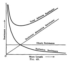
absorption loss is approximately proportional to the wave length. The effective resistance of the antenna or radiating circuit is the sum of the three components indicated above. It therefore varies with the operating frequency, as represented in Fig. 48, which also shows that this resistance passes through a minimum value for a given value of wave length, at which the sum of the three components is a minimum.
