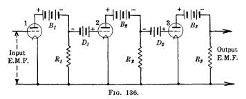
and its negative terminal to the resistance R, and choosing its potential equal to the potential difference across the resistance, will make the grid voltage of the second tube equal to zero.
