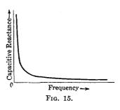
directly as the frequency due to the fact, stated above, that the rate of change of the voltage increases as the frequency.
