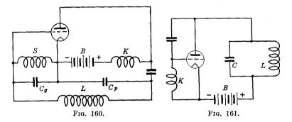
through the coil  $L_p$ , which may not be sufficient for sustaining the oscillations in the circuit LC. Thus, by suitably adjusting the capacity of the condenser H it is possible to regulate the amount of power fed back from the plate circuit into the oscillatory circuit LC. This constitutes, so to speak, an electrostatic control of the magnetic feed-back coupling of the plate and grid circuits.
