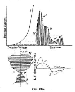
curve E, which is an exact reproduction of the envelope curve MNPQ, with its positive and negative halves of identical shape.
