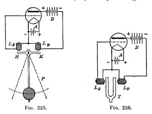
elasticity, in a manner similar to that of sustaining electrical oscillations. It is simply necessary that the mechanical system be started oscillating and made to vary the grid potential of the tube in such a way that the resulting plate-current variations are of suitable magnitude and phase to sustain the mechanical oscillations.
