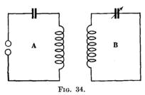
decreasing amplitude. Conditions in circuit B are thus the same as though an alternator were inserted in series with it, generating an electromotive force equal at every instant to the electromotive force actually induced by circuit A in circuit B. This was
