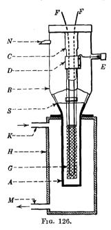
around the stem C, and to which is attached a connection wire coming out at E on the side of the glass cap, constituting the grid terminal of the tube. The nipple N serves to pump the air out of the tube when assembled, and is then sealed off in the usual way. When operating the tube, the cylindrical plate A is enclosed in a jacket or tank H filled with cold water, which is continually renewed through the pipes K and M in order to cool the tube.
