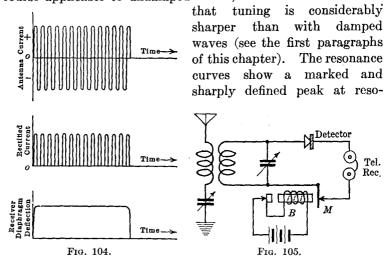
nance frequency, which thus greatly facilitates the elimination of interference from undamped wave sets of other frequencies.
