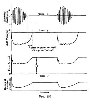
assumes the potential corresponding to zero current in its circuit. In the case of a tube free from all gas, as assumed here, this grid potential is zero. When the antenna circuit is then energized by incoming oscillations, say, a succession of damped waves emitted by a spark transmitting set, an oscillatory current is set up in
