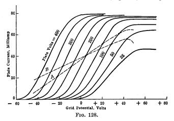
respectively to external plate circuit resistances R of 5,000 and 10,000 ohms, which crosses the successive static characteristic curves of the tube.
