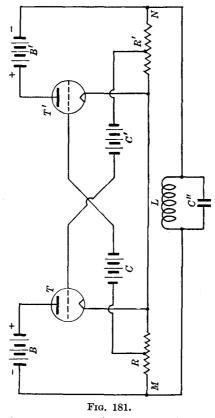
by itself until the power capacity of the tubes is reached. The minimum electromotive force required for such operation may be reduced by connecting the grids of the tubes to an intermediate point of the resistances R and R', as shown in Fig. 181.
