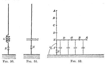
In order to change the wave length of a vertical wire antenna, it is then necessary to vary the length of the wire. Or an inductance coil L (Fig. 50), may be inserted in series with the antenna. This increases the total inductance of the circuit, and hence also
