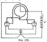
Radio Telegraph Transmitting Circuits.—Vacuum-tube oscillators as described above are widely used in undamped (continuous) wave radio telegraph transmission, for setting up high-frequency alternating currents in the antenna circuit. The methods used differ somewhat, however, depending on whether the apparatus is that of a stationary high-power station, or of a small low-power set, a portable field, or airplane radio set, for instance.
