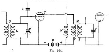
the electrons emitted by the filament to enter the grid circuit. Energy losses are thus created in this circuit, which absorb the excess of energy supplied by the tube, and prevent oscillation generation.
