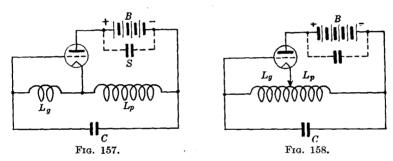
In all the above examples, the alternating component of the plate current flows through the battery B which furnishes the direct current to the plate circuit of the tube. In order to reduce high-frequency energy losses in the resistance of this battery, and also the disturbing effects of the electrostatic capacity between battery and ground, it is well to shunt the battery by a by-pass condenser, as shown in dotted lines in the diagrams.
