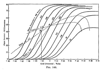
deg. out of phase, the ratio of these two electromotive forces is equal to
