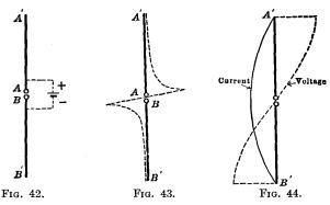
AA' will be positive and lose some electrons, while the lower wire BB' gains a like number of electrons and becomes negatively charged. This establishes a potential gradient along the system A'B', as shown in Fig. 43, where the deficiency or excess of electrons is plotted at each point of the wire A'B' perpendicularly to it. An electrostatic field is thus created about the wire, representing a store of potential or electrostatic energy.
