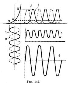
each other, as in Fig. 144, the output electromotive force is proportional to the *difference* of the two plate currents, and, as shown by curve 6 (Fig. 146) is a pure amplified reproduction of the input electromotive force: the device operates as a substantially distortionless amplifier.
