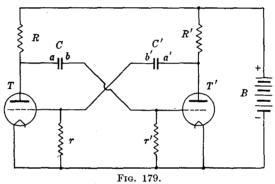
the grids of the tubes will suddenly be at the same potential as the filaments. This, in turn, produces a corresponding increase of the current in the tube T and decrease of the current in the tube T', so that the operation described above repeats itself in opposite direction.
