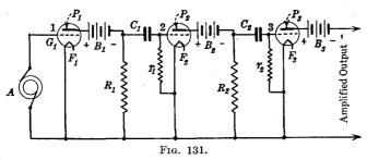
attracts during the positive cycle portions some of the electrons emitted by the filament. These in turn impart to the grid a negative charge which, increasing at every successive positive cycle portion, would soon stop the flow of current in the tube and prevent its operation.
