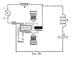
tudes and frequencies not higher than a few thousand cycles per second. It is therefore not suitable for radio transmission purposes, although the generated oscillations are very nearly sinusoidal.
