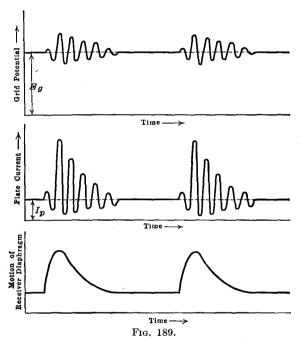
component, to a direct-current (rectified) component proportional to (or direct function of) the amplitude of the received signals, hence variable if these are damped or modulated, producing then a sound in the telephone receiver.
