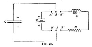
accumulating a negative charge on the upper condenser plate and a positive charge on the lower plate, as explained in a previous section. This charging current flows in the circuit until the electrostatic field created between the condenser plates by the charges on them exactly equals and counterbalances the battery electromotive force. The condenser being then fully charged, the amount of energy stored in it as potential energy is, as known,
