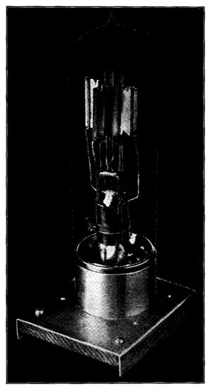
Plate 2.—Three-electrode vacuum tube used as high power oscillator and modulator. The plate has been forced downward to expose the grid and filament axially mounted. Note the cooling flanges on the plate. Signal Corps tube type VT-18.
