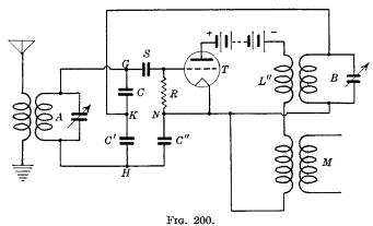
The arrangement may be considered as an alternating-current bridge circuit, the four corners of which would be points e, d, h, and F. The electromotive force, due to the incoming signals, is applied to this circuit system at points d and F; that, due to the locally generated oscillations, is applied at points e and h.
