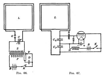
the secondary S of an induction coil, the primary winding P of which is energized by the battery B when the key K is closed, the primary current being rapidly interrupted by the vibrator V. The condenser D serves merely to quench the spark at the vibrator, and thus bring about a quicker break of the primary current.
