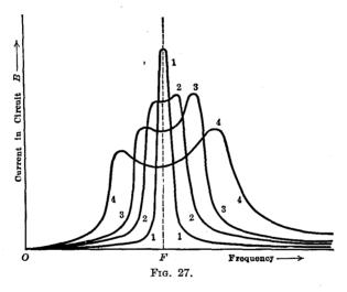
circuits, having individually a same resonance frequency and coupled not too tightly, will carry an appreciable alternating current over a band of frequencies, that is, at frequencies comprised approximately between the two resonance frequencies of the circuit-pair arrangement, which may hence serve as a frequency band filter.
