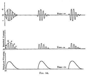
mitting set, while the frequency of the oscillations within each wave train is called the *radio frequency*.
