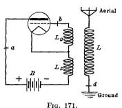
wide range of frequencies. The only adjustment then required is that of tuning the antenna circuit so that it will have a natural frequency equal to that which is to be transmitted. This is done by means of a variable inductance or capacity inserted in the antenna circuit. The key may be inserted at point a in the plate circuit, or b in the grid circuit, the opening
