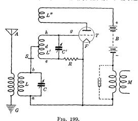
the grid g and may hence be considered as connected to the filament of the tube through the internal grid-to-filament resistance of the tube. The other side e of the coil L' and condenser C' is then connected to the filament F through a resistance R which is adjusted to be equal to the average value of this internal grid-filament resistance of the tube.
