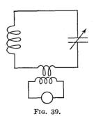
order to keep down the resistance of the wavemeter oscillatory circuit and thereby increase the sensitivity of the device by reducing the energy losses in it, the current measuring instrument may be loosely coupled to the circuit (Fig. 39) instead of being connected directly in it.
