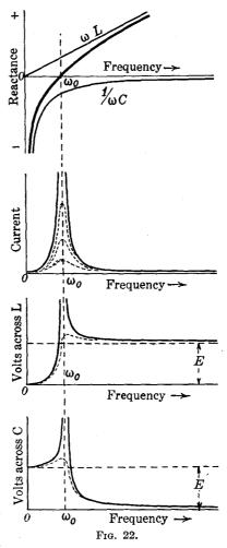
line curve in the diagram, is thus, at the smaller frequencies, of the nature of a large capacitive reactance. As the frequency increases, the value of this resultant reactance decreases until, for a given frequency  $\omega_0$  the inductive and capacitive component reactances being equal, the total reactance is zero. Thus,
