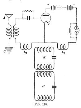
forms the feed-back coupling link or channel between the plate and grid circuits of the tube. The properties of this arrangement are distinctly different from those of the former, due to the fact that the oscillation-sustaining impulses are here transferred from the plate to the grid circuit through the medium of the currents in both circuits H and K.
