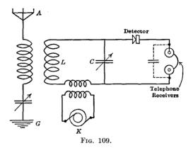
antenna circuit AG being tuned to the incoming waves, these induce a current of their own frequency  $f_1$  in the closed oscillatory circuit LC. This current may be represented by the upper curve of Fig. 108. As explained previously, this current when rectified by the detector would not produce a readable sound in the tele-
