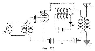
ferred to the antenna circuit depending upon the plate voltage of the tube, this is varied or modulated by connecting, in series with the battery B, the secondary winding of the transformer E through which the audio-frequency output electromotive force of the microphone circuit D is introduced into the plate circuit, adding to or subtracting from the battery voltage.
