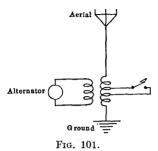
iron core carries a second winding connected in series with the key and with a direct-current generator. Closing the key then sends a direct current through this second winding, which partially saturates the iron core, changing its magnetic permeability and, hence, altering the value of the inductance and the tuning of the antenna. This principle is used
