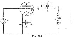
$1/\sqrt{LC}$  is equal to the cyclic frequency of the alternating electromotive force applied to the grid circuit of the tube. No alternating current will then flow in the plate circuit of the tube, and an alternating electromotive force  $ke_g$  will be developed across the circuit LC (and also between the filament and plate of the tube).
