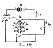
and coupled inductively to the grid circuit of the tube, as in the preceding example. Let M be the mutual inductance between the grid and oscillatory circuits, and assume for simplicity the resistance R of the oscillatory circuit to be all in the inductance branch of the circuit, the resistance of the condenser branch being negligible. Let  $i_L$ ,  $i_C$  and
