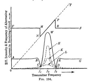
well-known resonance curve L (Fig. 194) is obtained, giving the current intensity in the circuit LL'C in function of the transmitter frequency f. At the same time, the frequency of the current in the circuit LL'C being always equal to the transmitter frequency, it is represented in function of the latter by the straight line OT (Fig. 194).
