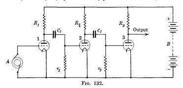
the advantage of being very simple to build in small and compact form, particularly as it may be arranged in such a manner that the plate circuits of all the tubes are energized by a single common battery B, while the filaments are heated from another common battery, as shown in Fig. 132, the plate circuits and filaments of the various tubes being simply connected in parallel across their respective batteries.
