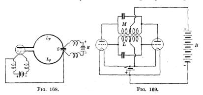
wires about 1 ft. long, the generated current has a fundamental frequency of the order to 80,000,000 cycles per second, and contains fairly strong second, third, and fourth harmonics.
