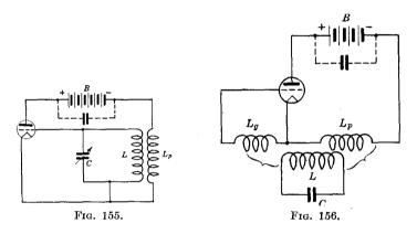
variations which in turn induce an electromotive force in the oscillatory circuit, which is in phase with and equal to (or greater than) the electromotive force operating in this circuit.
