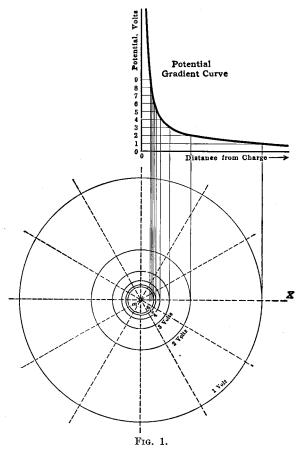
tron ring with respect to the positive atom center. This displacement of the component charges of the atoms represents a certain amount of work on the part of the electrostatic field of the charge m, and a consequent decrease of its potential energy, as explained in the preceding section, which correspondingly reduces the radii of the equipotential spheres representing the field of the charge m. In order to restore the field to the value
