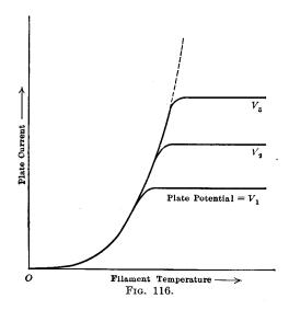
the electron emission from the filament, and, therefore, also the number of electrons present in the space of the tube. This group or cloud of electrons between the plate and filament produces a negative *space charge*, the effect of which upon the electrons leaving the filament is opposite to that of the positive charge on the plate.
