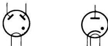
Fig. 2.1. Tube symbols (left: two-anode directly heated gas-filled rectifying tube, right: single-anode indirectly heated gas-filled tube).
