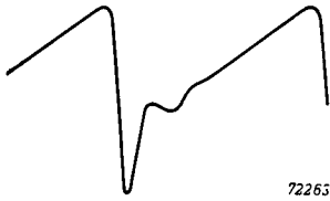
Fig. 4 Current in the deflection coils in the case of little damping.
