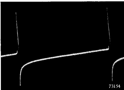
Fig. 55 Saw-tooth voltage at the grid side of the blocking transformer Type 10850. The peak-to-peak value is approx. 800 V, the positive peak at the start of the flyback is 420 V.
