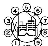
9FA 5BR8, 5FV8, 5MB8, 6BR8, 6BR8-A, 6FV8, 6FV8-A, 6JN8, 6MB8, 12EC8, 12JN8, 19HV8, 19JN8, 8446
