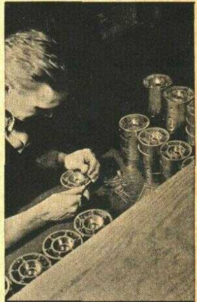
6 - ASSEMBLING ATTENUATOR HOUSINGS
