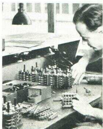
18 - ASSEMBLING FREQUENCY-CHANGE SWITCHES
