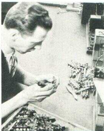
17 - INSPECTING SWITCH CONTACTS
